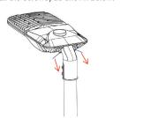
5. Rotate the lamp to a proper Angle (up to 20 degrees, down to 10 degrees), then tighten the two bracket screws, as shown below.
