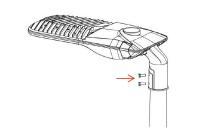
4. Unscrew the two screws of the bracket (do not unscrew all the screws) as shown below.
